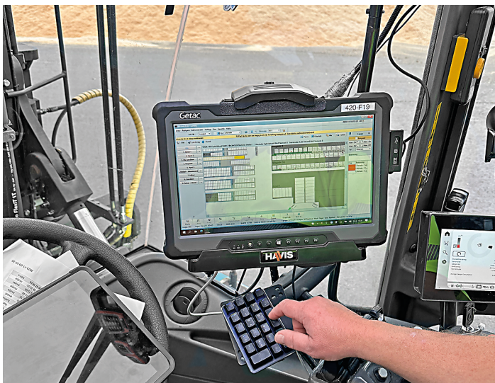
Picture 3: Forklifts are equipped with monitors, making it easy for drivers to visualize all the stock-locations, packages and open tasks.
