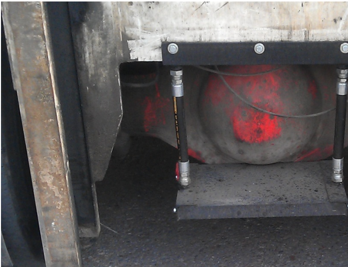
Picture 1: Forklifts are equipped with antennas. When picking-up or dropping-off packages, the antenna interacts with the transponders and locates the actual storage.
