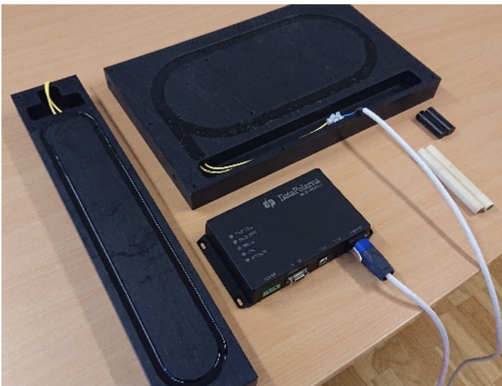
Picture 2: 2 types of antennas - mounted on forklifts, a RFID-reader (connected to antenna and computer in forklift) and 3 transponders (size as AA batteries). The transponders are positioned in the ground below every storage-space.
